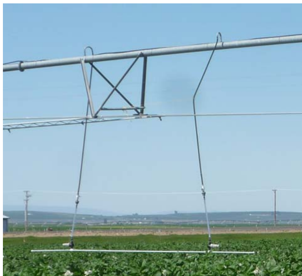
A new irrigation boom that decreases drift was discussed in relation to soil fumigation.
